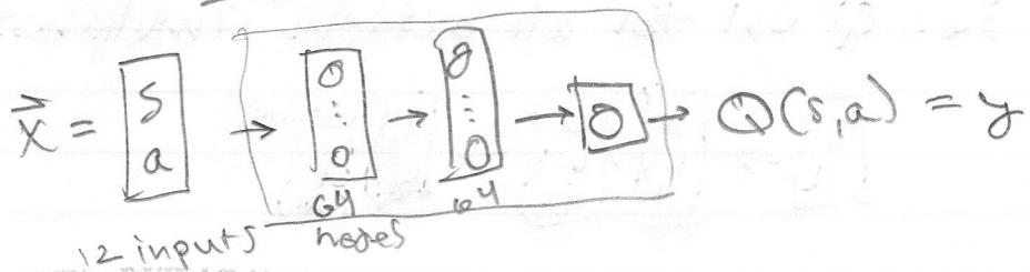
where  $s$  has 8 dims. and  $a$  is a one-hot encoding of  $a \in \{\text{nothing, L, R, main}\}$ .
